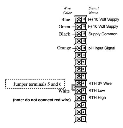
Figure 7-11 Terminal Designations for Durafet II Electrode with External Preamplifier
